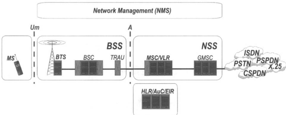
**Figure 2.2.** Basic GSM network and its subsystems
