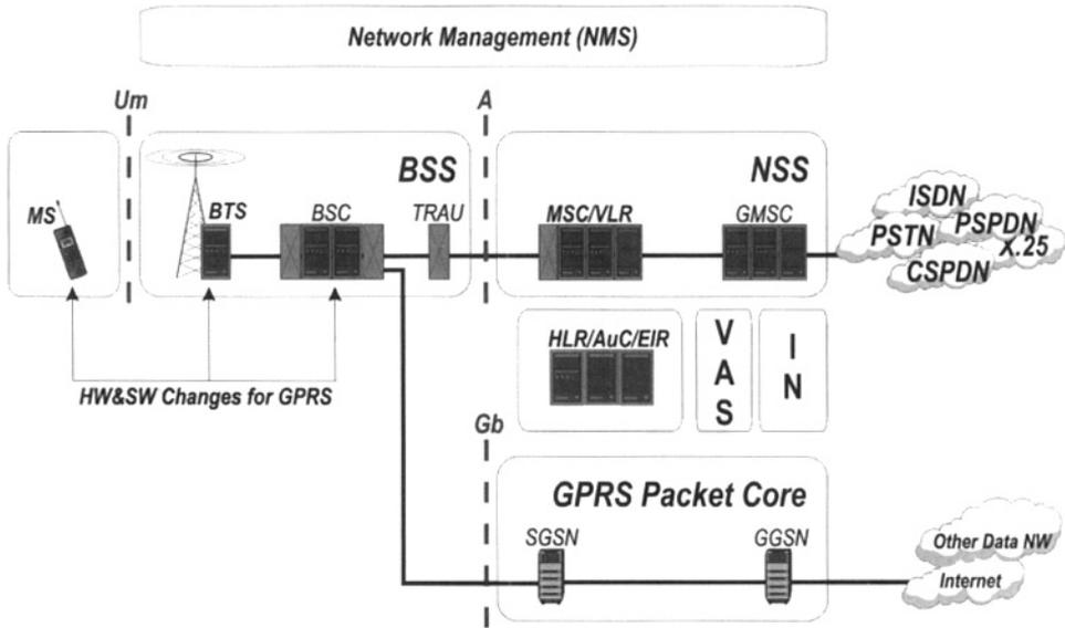
Figure 2.6. General packet radio service (GPRS)
