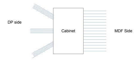
50 pair, 100 pair, 200 pair etc. multi pair cables are drawn from MDF to cabinet. From the cabinet 10 pair, 5 pair cables are drown up to Distribution Points (DPs). **Primary cable** - MDF to cabinet cable is called primary cable. **Secondary Cable** - Cabinet to DP cable is called Secondary Cable. Primary cable to Secondary cable jumpering is done at the cabinet.
