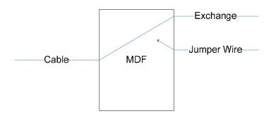
When a new connection is given the exchange side relevant point and cable side relevant point are connected by using another small cable. This small cable is called a jumper wire. MDF is a passive device. (No need of electrical power to operate.)
