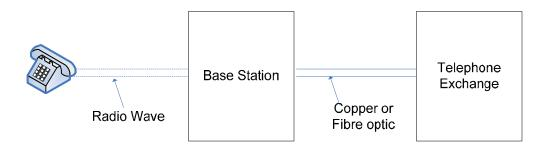
Telephone is connected to Base Station by using a radio wave. The Base Station is connected to telephone exchange by using copper or fibre optic.
